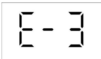
10.3 During self-cleaning process, if display screen shows the error code “E-3” when door is locked into place. It means that the door lock or detection circuit is faulty. When the error code appears, the buzzer will continuously prompt for 10 times (1s/time). If this error is shown, long press KB or K2 “⌚” key can return to standby mode.
