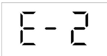
10.2 When the temperature is below <math>35^{\circ}\text{C}</math> after 5 minutes of heating (except for defrost mode, bottom heat element, fan gear and Eco mode), it means the heating element has a problem, the display will show E-2, the buzzer will prompt continuously for 10
