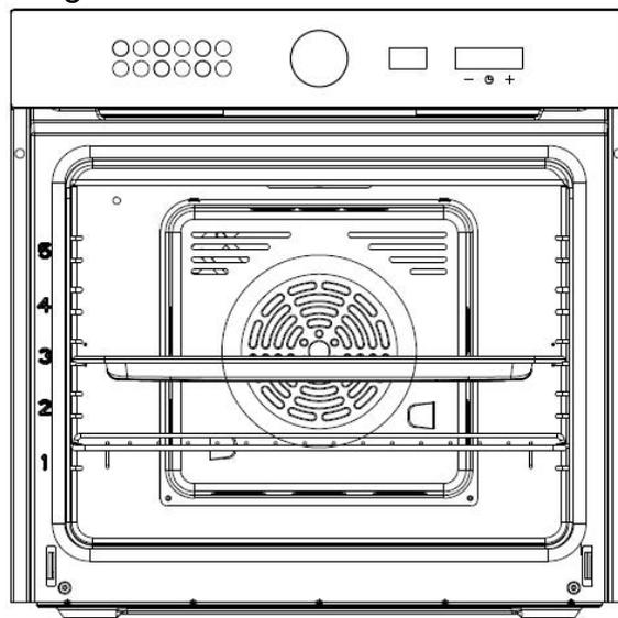
The accessories can be pulled out approximately halfway until they lock in place. This allows dishes to be removed easily.
