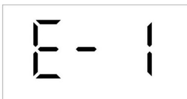
10.1 Display will show E-1 if the sensor is short circuit or open circuit under cooking mode, buzzer will continuously prompt for 10 times (1s/time), refer to display effect 11. Oven will be locked at this time, at this time long press KB or K2 "🕒" key can return to standby mode.(Cooling fan will keep working)
