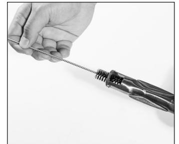
**STEP 04** Brush entire outer surface of burner to remove grime.
