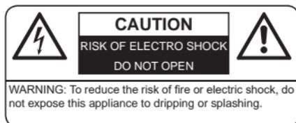
WARNING: To reduce the risk of electric shock, do not remove cover (or back). No user serviceable parts inside. Refer servicing to qualified service personnel.
