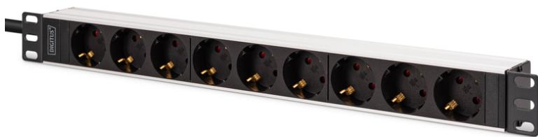
**1U Alu PDU, rackmount, 8x Safety outlet, 1x outlet 16A, 230VAC, 50/60Hz, IEC C20 Stecker**
