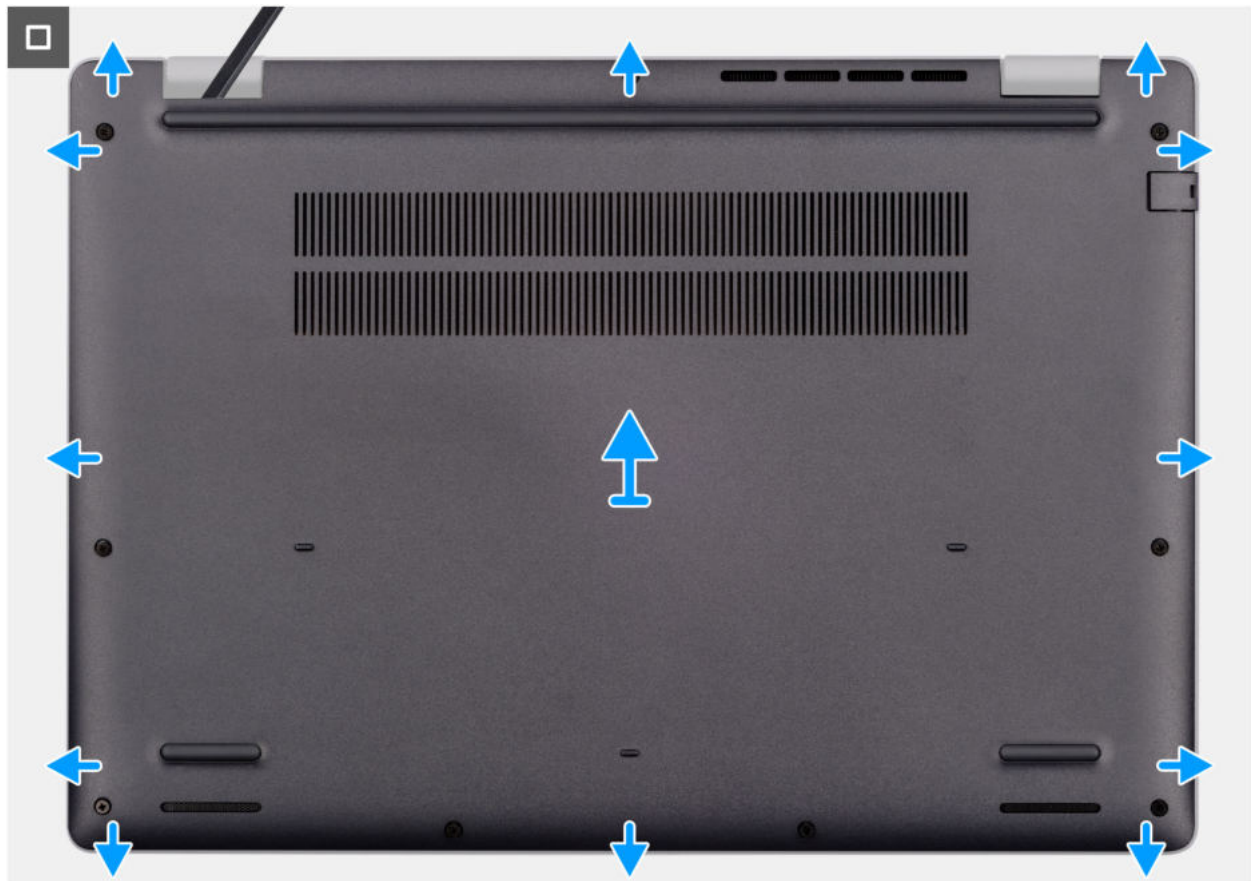
Abbildung 12. Removing the base cover
