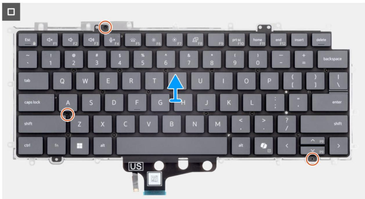
Abbildung 96. Removing the keyboard
