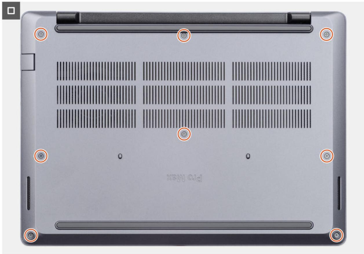
Abbildung 15. Installing the base cover
