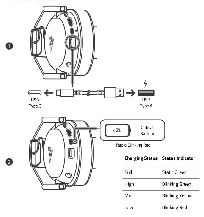
For best results, connect your Razer BlackShark V3 X HS directly to your computer's USB port using the provided cable. A depleted battery will be fully charged in approximately 4 hours.
