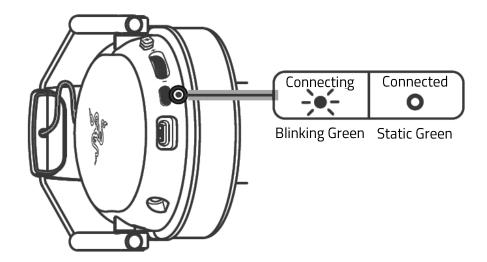
Customize the LED indicator to show the headset's connection status, battery status (default) or low battery warning using Razer Synapse.
