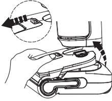
Press the Clean Water Tank release button to remove it from the appliance.
