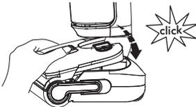
Place the tank back into the appliance. You should hear a click if done correctly.
