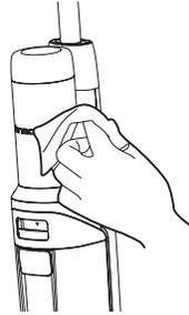
Use a cloth to clean the surface with a neutral detergent. The cloth should be dry to prevent water from entering the appliance.
