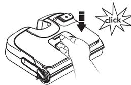
Place the tank back into the appliance. You should hear a click if done correctly.
