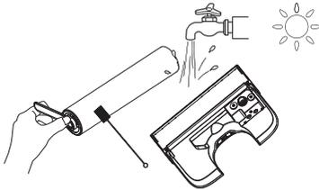
Use the cleaning tool to remove hair and debris wrapped around the roller and rinse the roller and back of the CWT with water. Allow them to dry completely before reinstalling.
