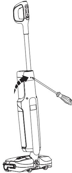
In the event that the handle needs to be disassembled, press the spring to release the handle with a tool (like a screwdriver) and lift the released handle from the appliance.
