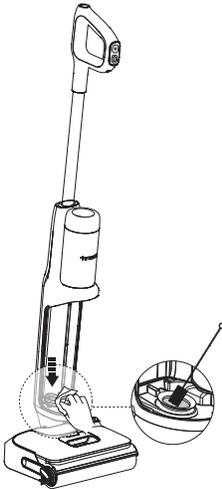
Clean the dirt sensor with a damp cloth or the cleaning tool.
