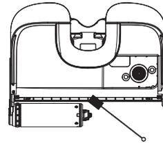
Remove hair and debris from the brush roller chamber and the opening with the cleaning tool.
