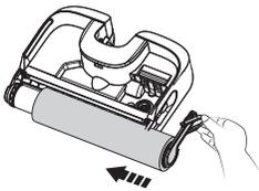
Replace the brush roller by inserting its end into the left side of the holder, then attach the roller tab to the magnetic buckle on the right side to lock into place.
