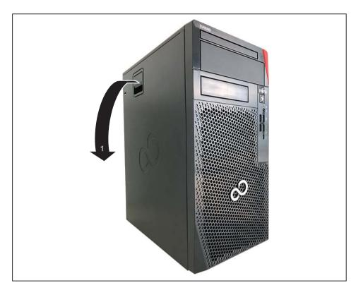
▶ Pull the latch and lift the side panel off the housing (1).
