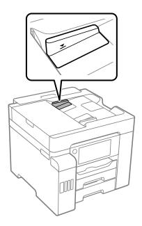
The original slips when paper dust adheres to the roller.
