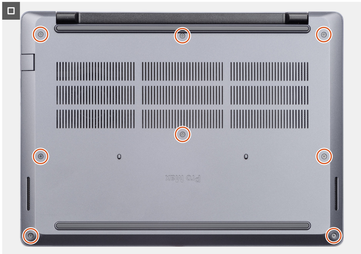
Abbildung 15. Installing the base cover
